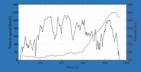
In RDE tests, several new contributions can be identified impacting on the on-road measured emissions, as example:
